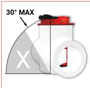
**FIG. D: SENSOR TILT THRESHOLD**
