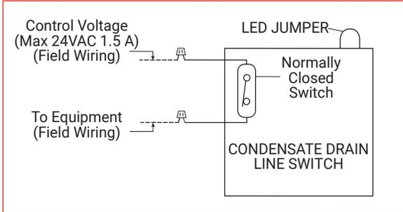
FIG. E: WIRING DIAGRAM
